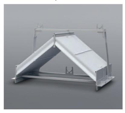
Munters DV210+ is a V-shaped vane type separator system for vertical gas flows. The system is typically used in gas cleaning devices such as flue gas desulphurization absorbers and wet scrubbers.
