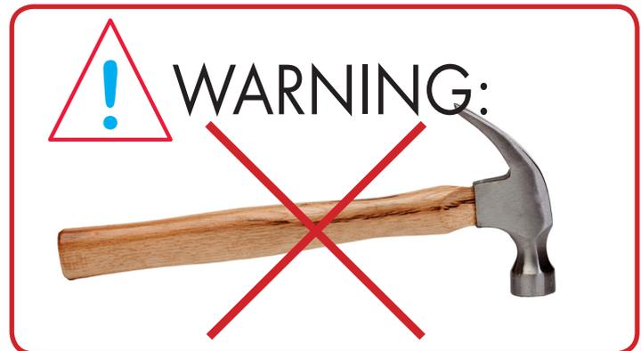
**DO NOT** use metal hammer to secure the MWI. The use of a metal hammer can result in damage to MWI.
