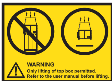
Figure 1.3 Lifting of unit not permitted.
