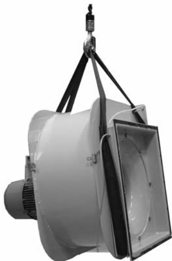
Figure 3.12 Lifting the reactivation fan
